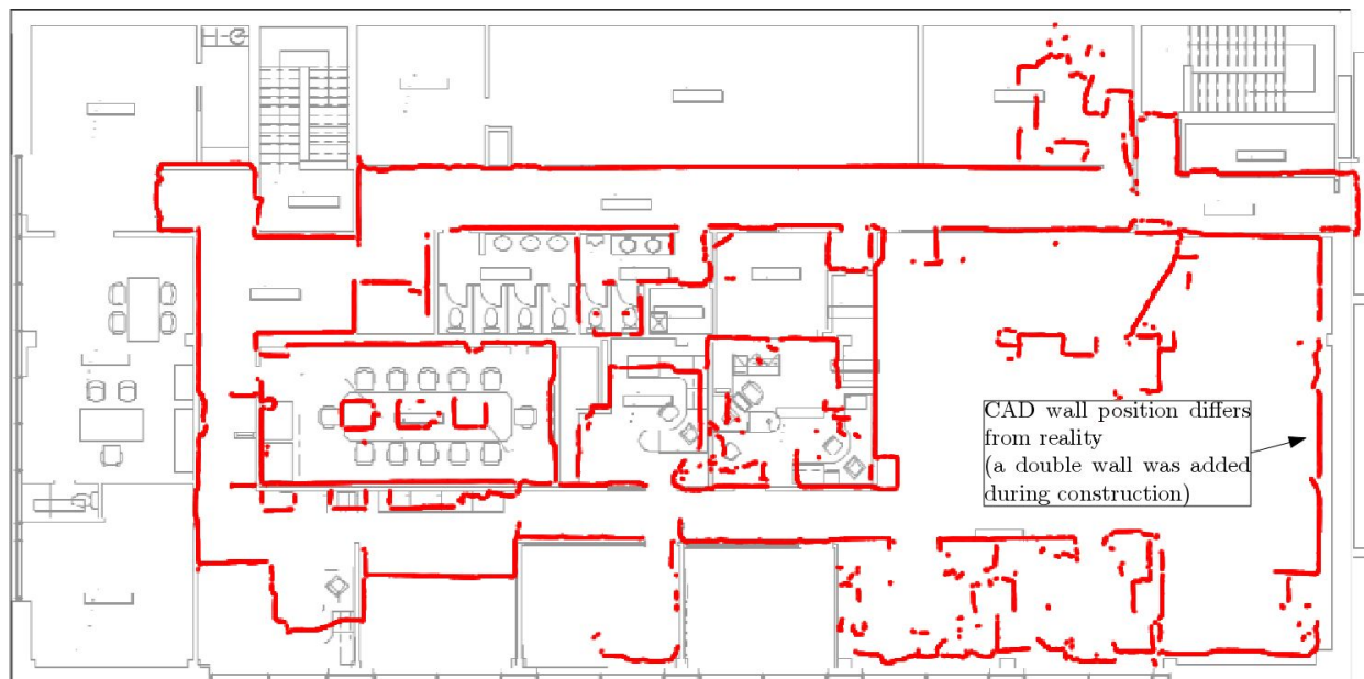
Figure 4 : Closeup example of a map created by the robot superimposed over the CAD of the building.
