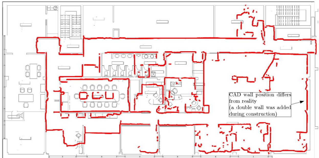
Figure 1 : Building's CAD error detection through robot 2D scanning
